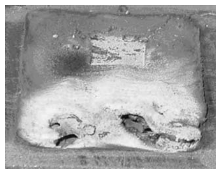
Fig. 20 Result of SLS with an uncontrollable SHS reaction. In the center it can be clearly seen the square area, in which sintering was proposed. Regime treatment corresponds to Fig. 13. Comments the same as for
