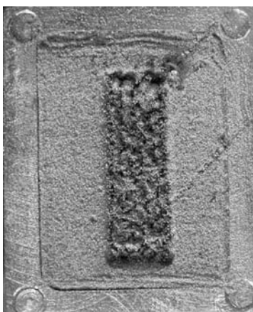
Fig. 19 Sintered monolayer of powder mixture Ni–Ti=1:1. Regime treatment corresponds to Fig. 6. Comments the same as for Fig. 18
