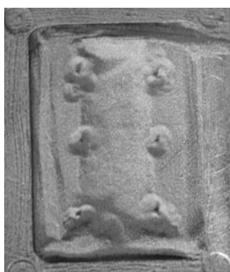
Fig. 3 Appearance (top) of cuvette for sintering of powders, pointers shows the thermocouple places
